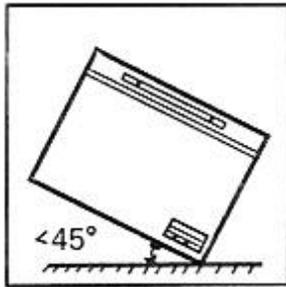
1. When you transport the freezer, the angle between the compartment body and the ground should be no more than  $45^\circ$ , and you should never place the freezer up-side down.
