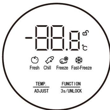
1. When powering up for the first time, perform self-test (all LEDs on the display panel are on for 1 second, off for 1 second), and the self-test ends to enter the setting state. The button is unlocked, and the display screen flashes (unlocked state) to display the current setting temperature. The default setting temperature of freezer is -18.0 °C.
