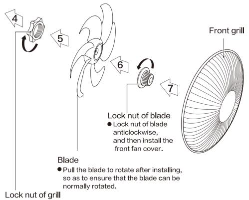
• Screw the lock nut of grill clockwise, and in the meantime, fix the rear grill.
